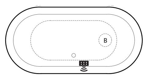
Airbath System II Blower must be remotely located (Diagram is required for custom blower connection locations)
